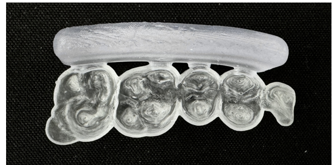
Figure 16: Single-sided MouthIO brace. The braces are only attached to one side of the molar teeth which leaves the front teeth free. This might avoid lipping as the front teeth are not covered with the braces.
