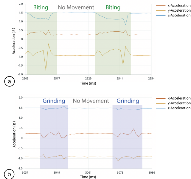
Figure 11: (a) Data showing acceleration patterns between biting and no movement captured while wearing MouthIO, (b) and acceleration patterns between grinding and no movement.
