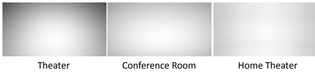
Figure 8: Calibration masks used to equalize the brightness across each screen.
