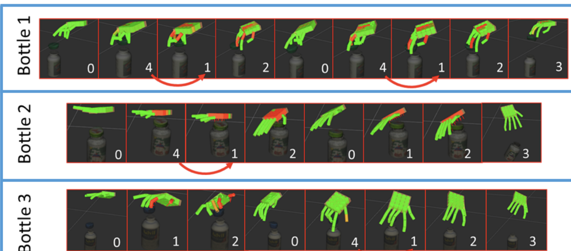
Fig 4. Key frames of opening various bottles with T-AOG. Numbers on bottom right indicate the cluster labels and the red arrows indicate the merges triggered by the parsing of T-AOG.
