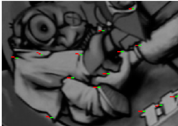
Figure 2.4: A typical example of the prediction of the next positions of the keypoints using gyroscope readings (Red lines are drawn between the initial position of a point and the predicted position while green lines are between the predicted position and the final position)
