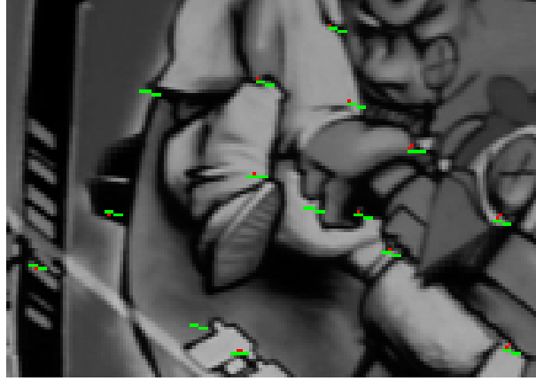
Figure 2.6: Worst-case scenario for the prediction of the next positions of the keypoints using gyroscope readings (Red lines are drawn between the initial position of a point and the predicted position while green lines are between the predicted position and the final position)
