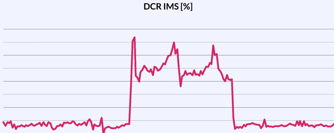
This graph shows a snapshot of this event where a problem with a single network element - a so-called media processor - out of about a dozen caused a rising DCR, affecting thousands of subscribers.
