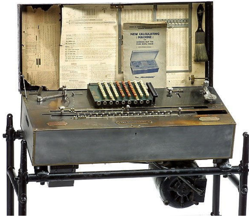
The Millionaire with the servo motor, ca. 1910 (© John Wolff)
