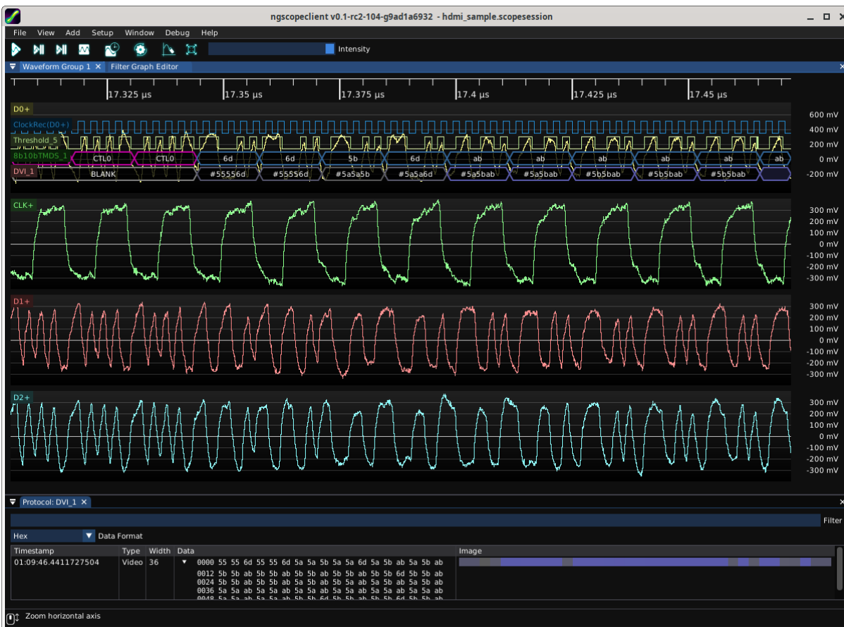
Figure 26.61: Example of decoding a DVI signal
