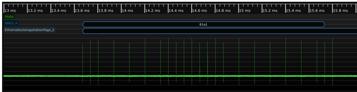
Figure 26.70: Decoding a single 16-bit link code word
