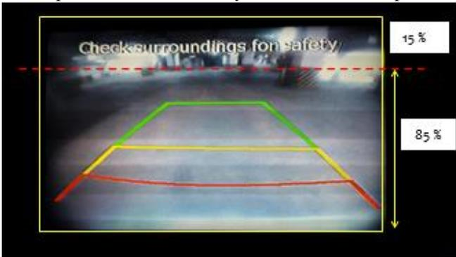
Horizon height of 85% from the bottom of IRVM LCD screen for a distance of about 100m.
