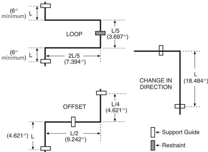
When installing an expansion loop, no rigid or restraining supports should be placed within the leg lengths of the loop. The loop should be installed as closely as possible to the mid-point between anchors. Piping support guides should restrict lateral movement and direct axial movement into the loop. Lastly, the pipe and fittings should be solvent cemented together, rather than using threaded connections.
