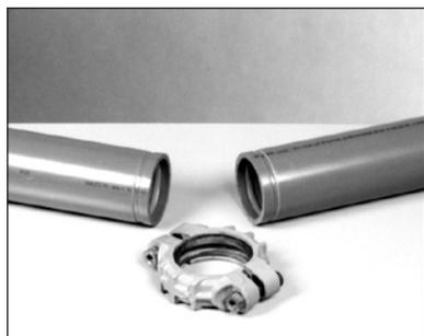
Check the pipe ends for any damage, roll marks, projections, or indentations on the outside surface between the groove and the end of the pipe. This is the sealing area, and it must be free of any defects.
