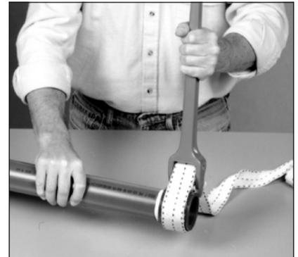
**NOTE:** Charlotte Pipe does not recommend threading any other thermoplastic pipe other than CPVC and PVC Schedule 80.
