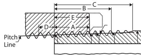
\*Per ANSI/ASME B1.20.1 and ASTM F 1498
