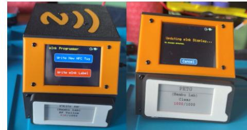
The software was written in Arduino's IDE with the help of AI (Gemini). I broke down each feature into a sprint, and made one change at a time, even when the AI would make multiple changes. While I did need to do some manual debugging and fixes this was very successful. The full code is on GitHub <https://gist.github.com/InsiderPhD/7ee1b9af25f642013b135f43f7a5f84b>.
