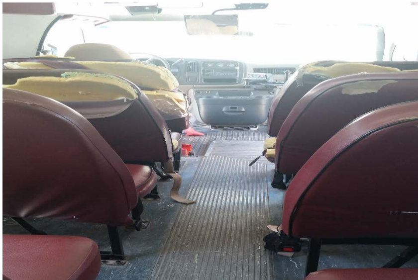
Photograph 4: Extremely worn and damaged bus seats.
