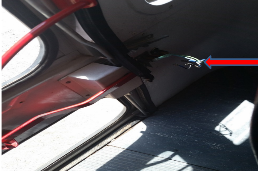
Photograph 5: Exposed wiring at rear exit door of van.
