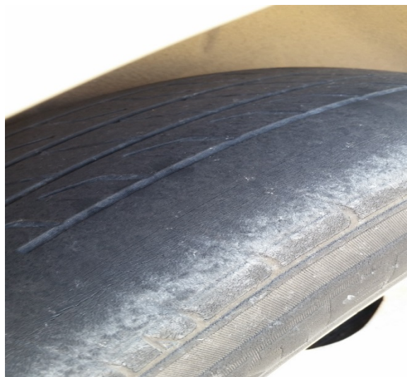
Photograph 1: Low tire tread on vehicle used to transport children.
