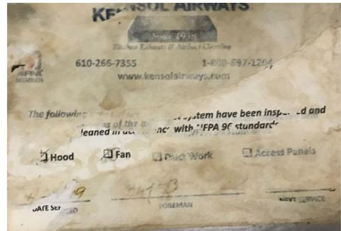
**Photograph 9 (left):** This fire extinguisher did not have any recorded monthly inspections. **Photograph 10 (middle):** This sprinkler head was obstructed by stored items; an 18-inch clearance is required for all sprinklers. **Photograph 11 (right):** As indicated by this inspection tag, the most recent kitchen hood inspection was in 2019, 2 years prior to our audit and with no next service date scheduled.
