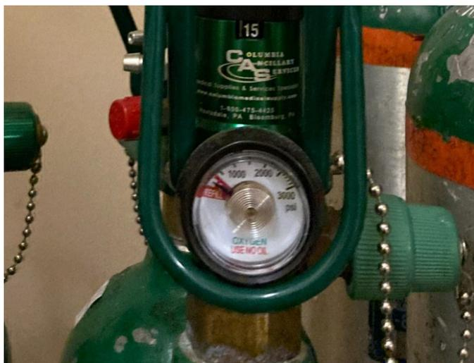
**Photograph 14 (left):** Empty oxygen cylinders were left in the "full oxygen cylinders" area. **Photograph 15 (right):** This close-up of the oxygen cylinder gauge from Photograph 14 shows that the gauge indicated that the oxygen cylinder was empty.
