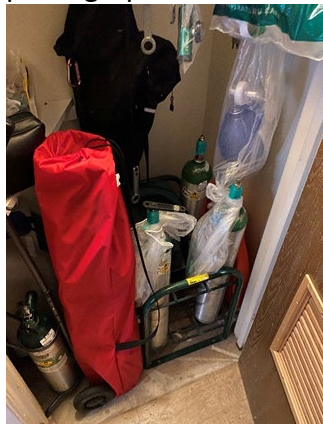
Photograph 5: Stored oxygen tanks were not clearly distinguishable as full or empty.
