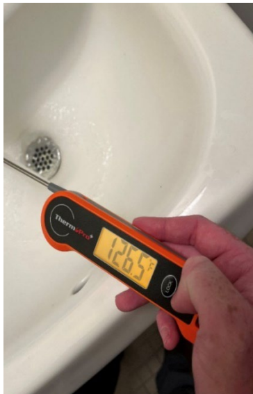
Photograph 7: All-purpose thermometer registering a water temperature of 126.5° Fahrenheit.
