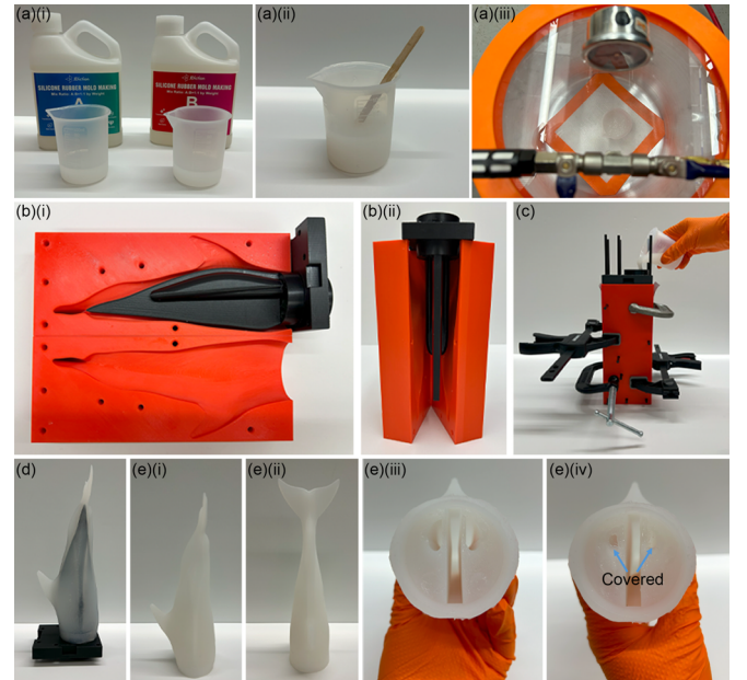
Fig. 3. Silicone Tail Molding and Demolding Process: (a) Molding steps: (i) Measuring silicone solutions, (ii) Stirring the mixture, (iii) Vacuum chamber treatment; (b) Mold preparation: (i) 3D-printed mold components, (ii) Pre-assembled mold; (c) Pouring silicone into the mold. Demolding the Silicone Tail: (d) Tail during demolding; (e) Final views of the tail: (i) Left view, (ii) Front view, (iii) Side view showing the two air chambers, (iv) Sealing the air chambers for waterproofing and buoyancy.
