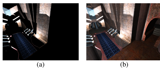
Figure 1: The Indirect Lighting Impact (a) presents a snapshot of Q3tourney2 (courtesy of Id Software) with direct lighting only (two point light sources). The screen resolution is 1024 \times 768 . (b) The same scene with 512 secondary point light sources. Using interleaved deferred shading, the scene is rendered at 17 f/s on a GeForce 6800 GT and 33 f/s on a NVidia GeForce 7800 GT.
