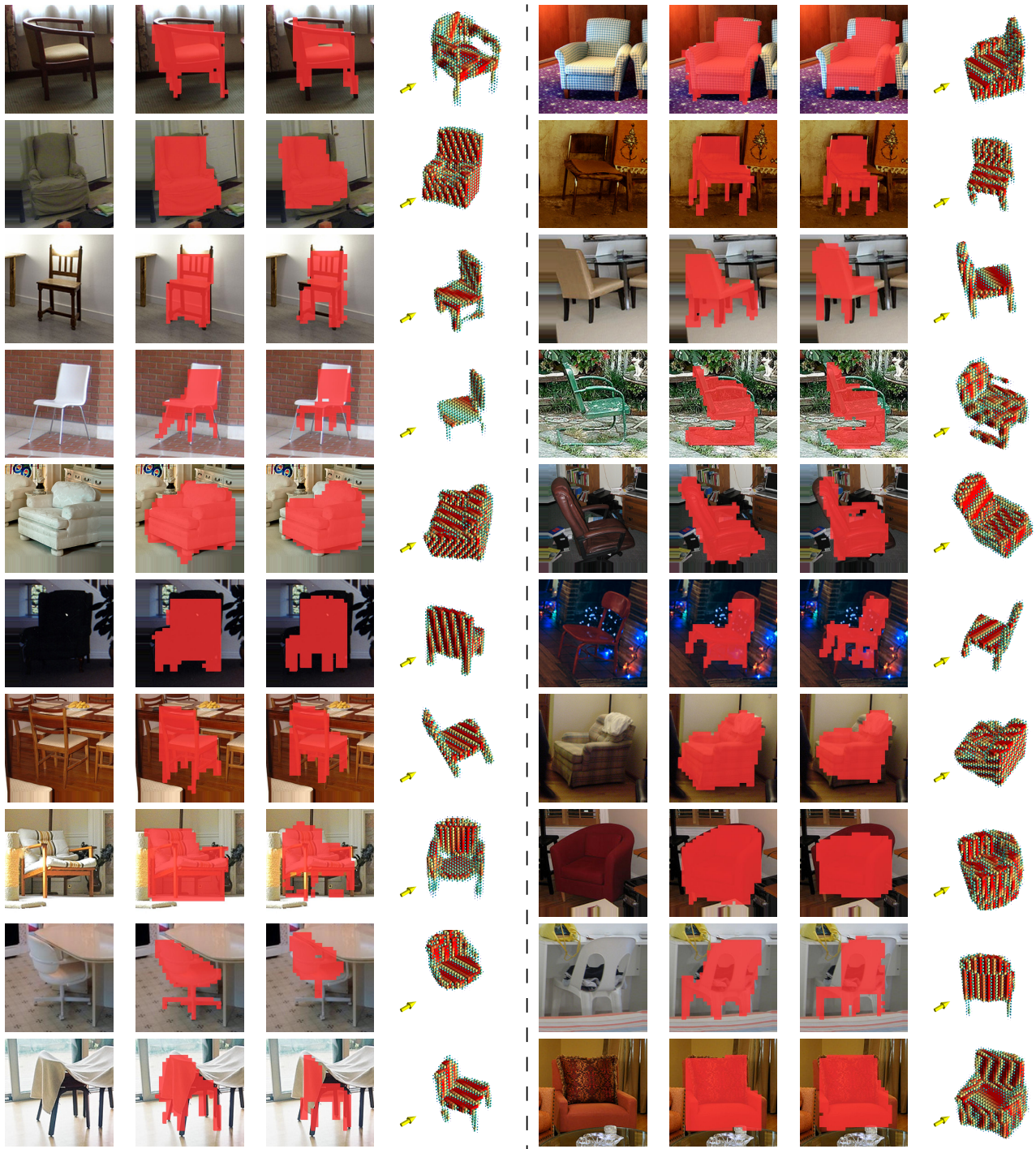
Figure 3: Reprojected silhouette as instance segmentation (chair). For each sample we show the input image (left), ground truth segmentation (middle left), reprojected silhouette (middle right), and reconstructed pose-aware shape (right).
