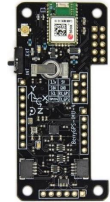
Figure 32: BerryGPS-IMU GPS and 10DOF
