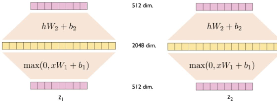
In addition to attention sub-layers, each of the layers in our encoder and decoder contains a fully connected feed-forward network, which is applied to each position separately and identically. This consists of two linear transformations with a ReLU activation in between.
