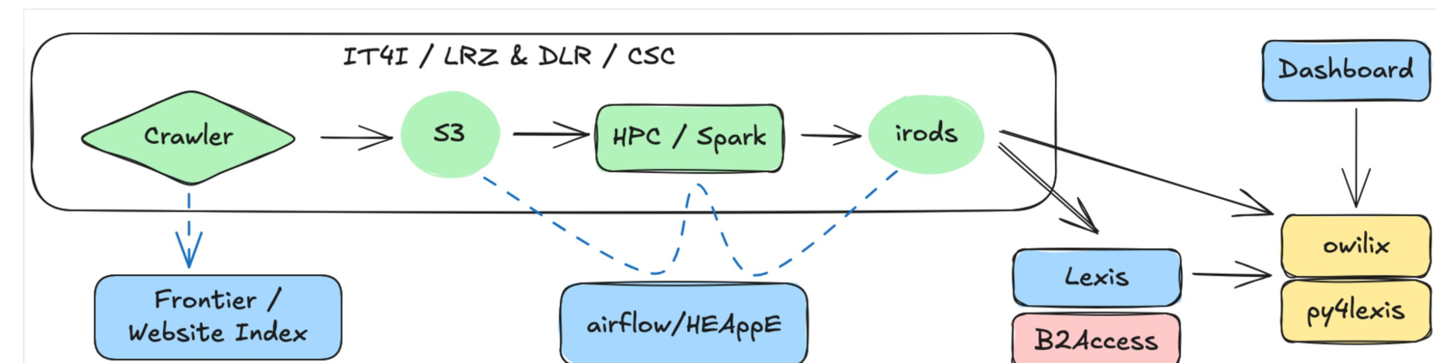
The OWS processing pipeline consists of large-scale web crawling, preprocessing, index generation, and dataset publication. These workflows are executed across major European HPC centers, including IT4Innovations (CZ), Leibniz Supercomputing Centre (DE), and CSC (FI). Parallel execution enables high-throughput processing of web-scale data.
