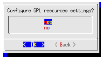
Figure 7.6: Slurm With cm-wlm-setup: GPU Configuration Entry Screen
