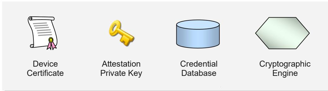
The *Device Certificate* forms together with a matching *Attestation Private Key* the foundation for the session mechanism that facilitates secure provisioning of keys, also when the provisioning middleware and network are non-secure.
