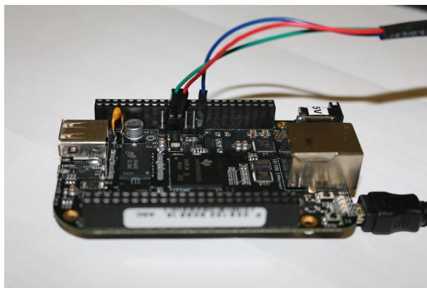
Once the USB to Serial connector is plugged in, a new serial port should appear: `/dev/ttyUSB0`.
