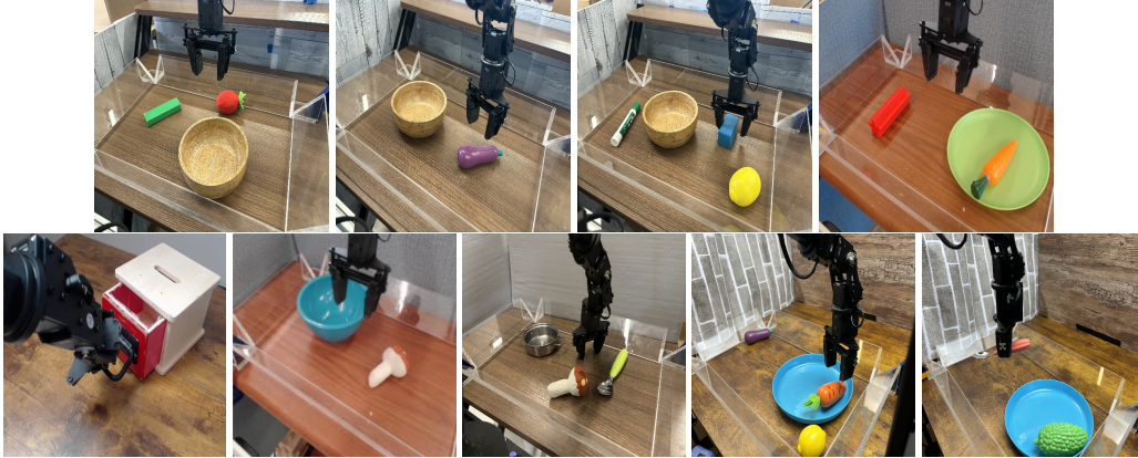
Figure 4: Across the five unique robot workspaces for the five WidowX robots, there are 9 different scenes, each scene corresponding to a distinct set of manipulatable objects available, and each scene supporting many different tasks that can be executed. 8 scenes support pick-and-place tasks, and 1 supports drawer opening and closing tasks.
