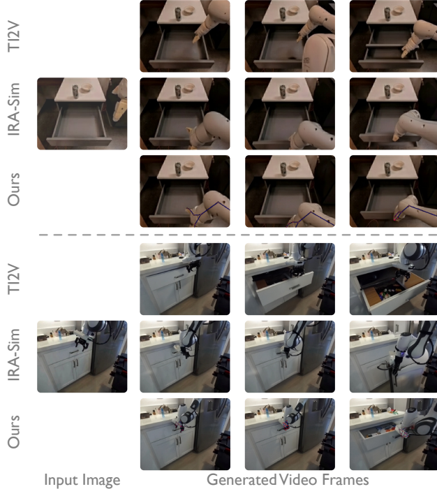
Figure 4. Comparison of different action control signals. Text as action (TI2V [72]) leads to ambiguity. Raw 7-DoF states/actions (IRASim [81]) leads to inaccurate control. Visual action prompts (Ours) facilitate dynamic learning under precise control.
