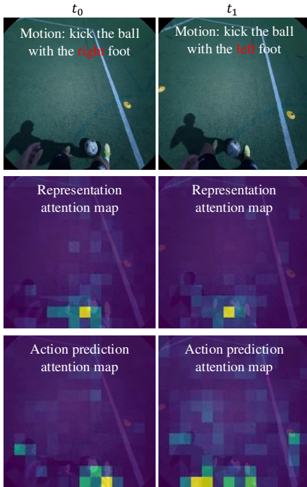
Figure 4. Attention map of EgoAgent performing visual representation and action prediction task. EgoAgent attends to the moving body part in the image when predicting future actions.
