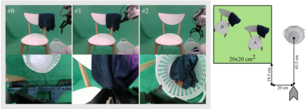
(e) Place Jeans to Basket: The robot base ( F_R ) is fixed relative to the laundry basket. The jeans is semi-folded and hanging on the right edge of the chair. The chair position is randomised in the 20\text{ cm} \times 20\text{ cm} region. The robot grasps the jeans from the side and places it in the laundry basket. We collected 50 demonstrations, in each half of the demonstrations the chair position is randomised keeping the orientation A and in the other half the orientation of the chair remained B. The average length of the demo is 592 steps or 44 secs.
