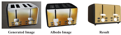
Figure 8: Failure case. Because of the unusual light effects generated by diffusion (silver metallic with yellow light), the albedo estimation network fails to accurately estimate the albedo, leading to dissimilar material prediction.
