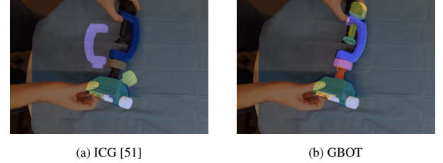
Figure 11: Tracking with assembly-state-graph in a real scene: We extend our assembly-aware tracking based on work of MbICG [50]. The introduction of assembly state graph helps improve tracking accuracy considering assembly constraints.
