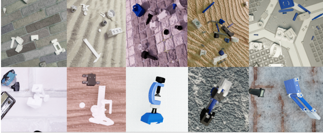
Figure 5: Our synthetic training images. Clustered scenes with 3D printing parts for the assembly parts are generated. To add domain randomization, we add objects from the T-less [20] dataset, varying lighting conditions, and randomized backgrounds.
