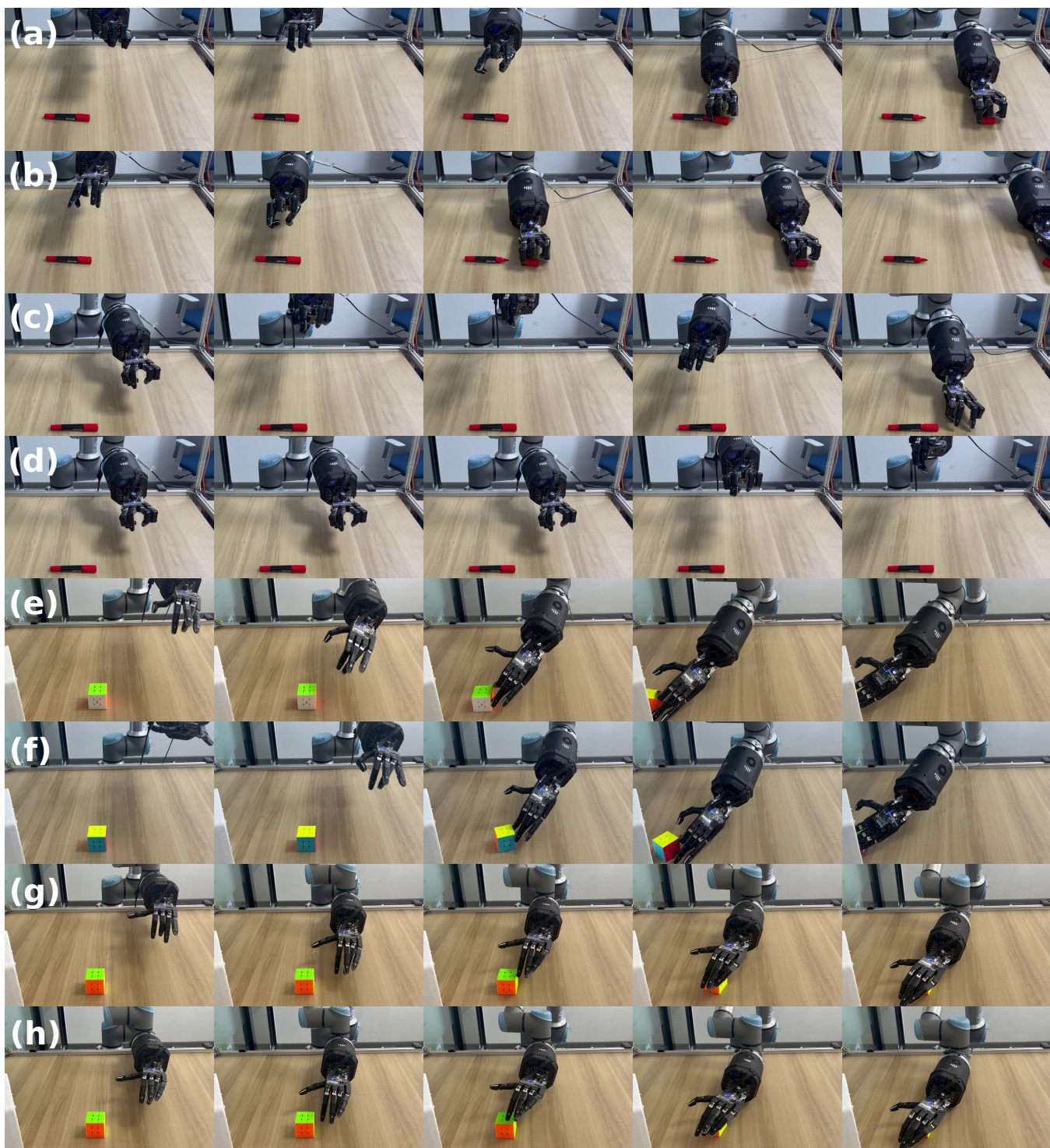
Fig. 21: The figure displays the trajectories of simulation-to-reality experiments with RM fine-tuning (ours) and vanilla policy training (baseline) on two tasks Pen and Relocate. [a-d] are Pen and [e-h] are Relocate. [a-b] and [e-f] are results by our method while [c-d] and [g-h] are the baseline results. From left to right it shows the procedure of the task completion.
