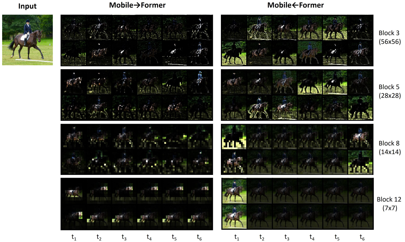
Figure 8. Visualization of the two-way cross attention: Mobile→Former and Mobile←Former . Mobile-Former-294M is used, which includes six tokens (each corresponds to a column). Four blocks with different input resolutions are selected and each has two attention heads that are visualized in two rows. Attention in Mobile→Former (left half) is normalized over pixels, showing the focused region per token. Attention in Mobile←Former (right half) is normalized over tokens showing the contribution of different tokens at each pixel. The cross attention has less variation across tokens at high levels than low levels. Specifically, token 2–5 in the last block have very similar cross attention. Best viewed in color.
