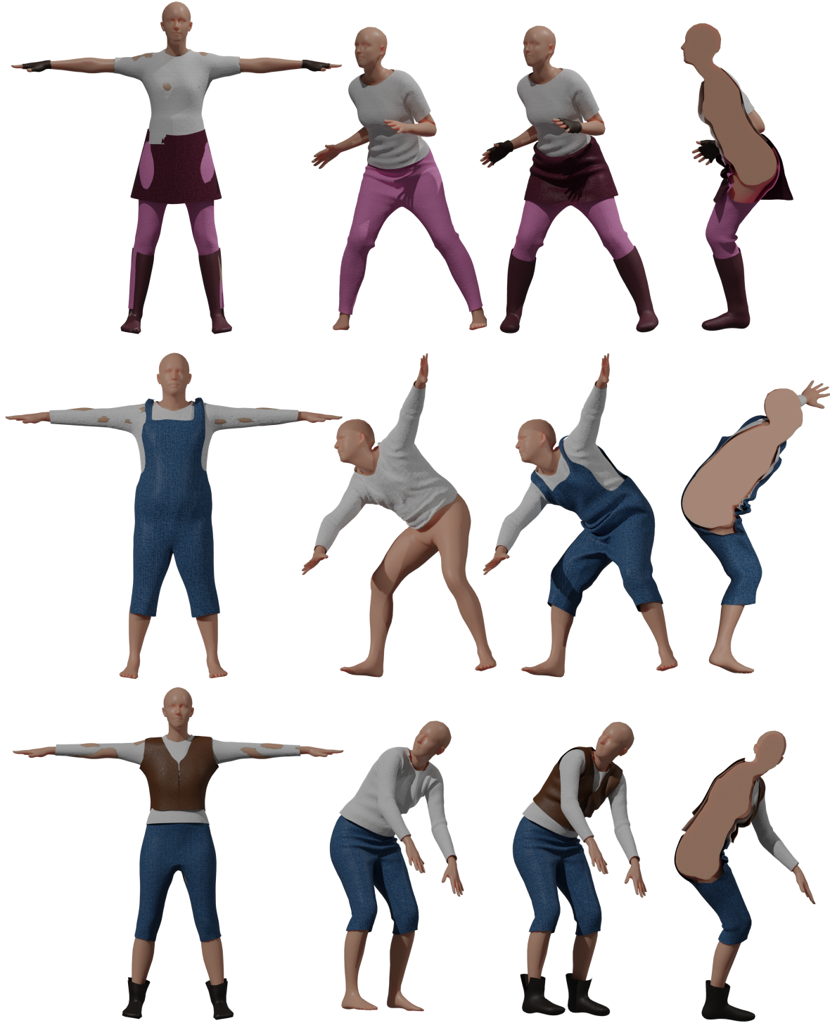
Figure 7: PBNS results on outfits with overlapping layers of cloth. Each row shows a sample. From left to right: template outfit, posed sample without outermost layer, posed sample with whole outfit and cross section. The proposed collision loss can handle multiple layers of cloth, even when the template outfit presents inter-penetrations. As we can observe on the cross section, PBNS is able to generate consistent predictions with minimal layer spacing. Also note how it is possible to neurally simulate different fabrics –different wrinkle count and size– within the same outfit by assigning per-vertex weights to cloth related losses.
