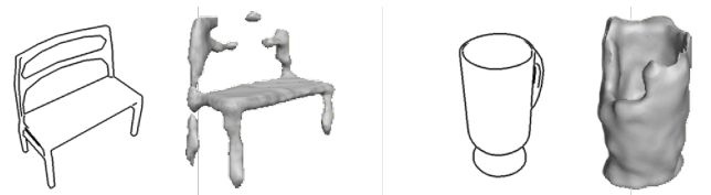
Figure 19: Thin structures are challenging to capture by the 64^3 voxel grid.
