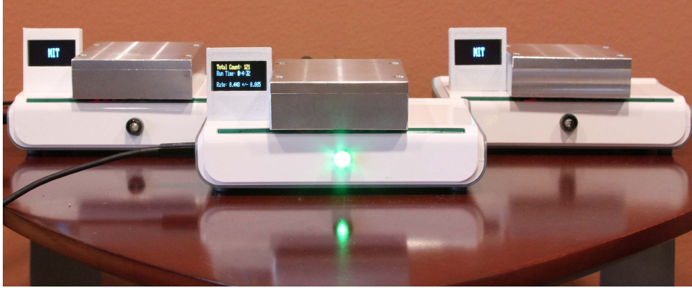
FIG. 1: An array of desktop muon detectors. When a muon passes through one of the aluminum boxes, the electronics box registers the event and displays the information on the OLED screen. The green LED in the front flashes for a period governed by the amount of photons absorbed by the photo-detector. The data can then be transmitted to a computer via a mini-usb cable.
