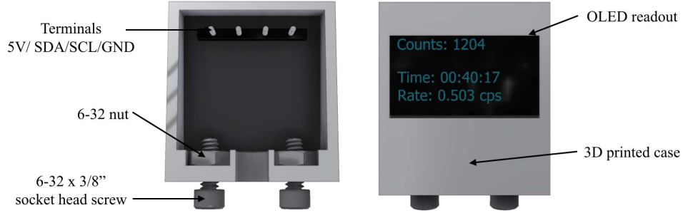
FIG. 6: Front and back view of the 3D printed OLED screen case.
